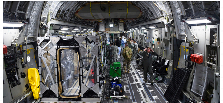
The TIS is an enclosure the Department of Defense can use to safely transport patients with highly contagious diseases. (U.S. Air Force photo by Senior Airman Cody R. Miller)
